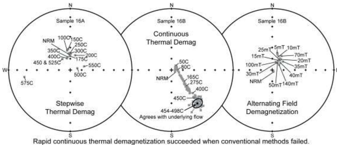
**Figure 1:** Comparison of three demagnetization methods on sister samples of Steens Mountain basalt
